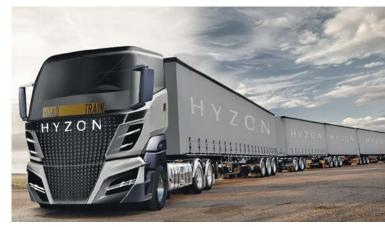
A Hyzon Motors fuel cell truck in road train configuration. Image: Hyzon Motors
